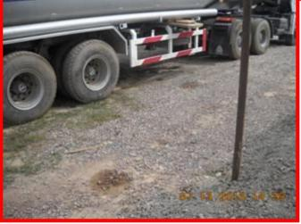
Photo No. 20: Diesel spills at the fuel refilling area
