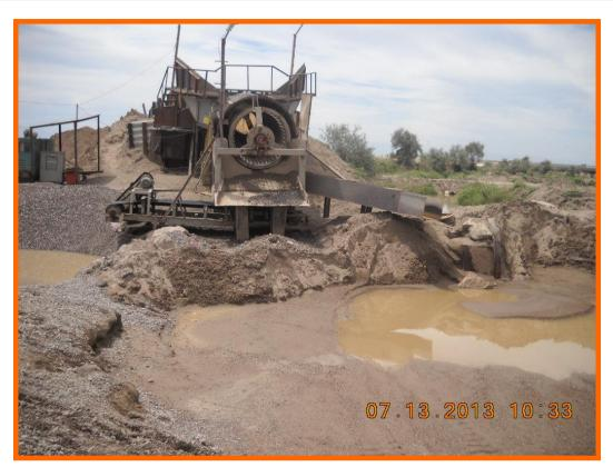
Photo No. 1 : Gravel and sand washing equipment
